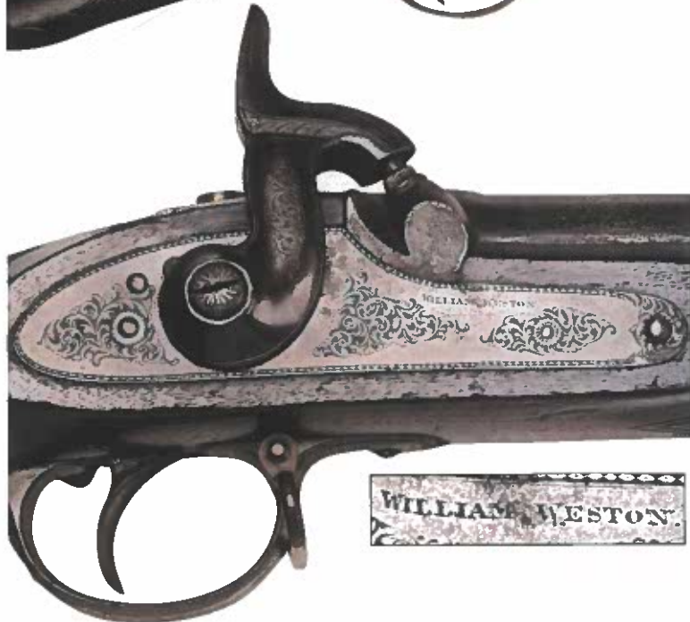
The lock of a high quality Pattern 1853 Volunteer rifle musket made by William Weston. Note the flower head engraving on the hammer screw that is found on all screws of the rifle.
