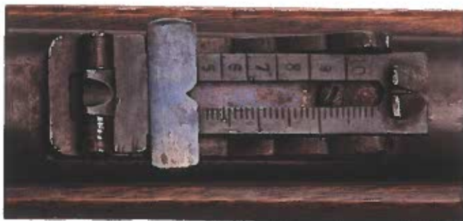
A vertical view of the unusual backsight found on most of the 40-inch barrel rifle muskets. Note the numerals are on the left side of the ladder rather than the right side as normally found.
