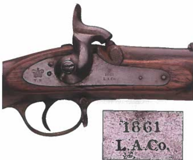
A typical, plain LAC lock without threads with a crown / "V.R" behind the hammer and "1861" / "L.A.Co." in front of the hammer.
