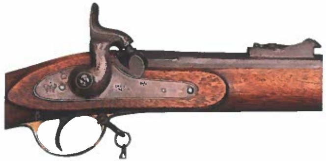
The lock area of a diverted Spanish Contract rifle musket with a distinctive part hexagonal section at the breech and unusual backsight.
