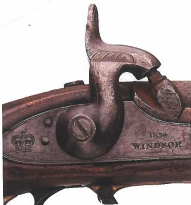
Pattern 1853 rifle musket lock, Type II made by Robbins & Lawrence of Windsor, Vermont under contract to the British Ordnance.
