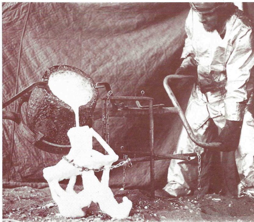
A brilliant orange in the molten state the 2100°F bronze is poured into the mold through a system of gates.
