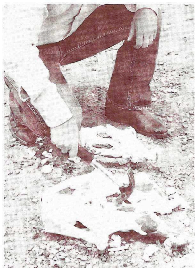
Taking many hours to cool, the bronze sculpture is finally broken out of the mold.
