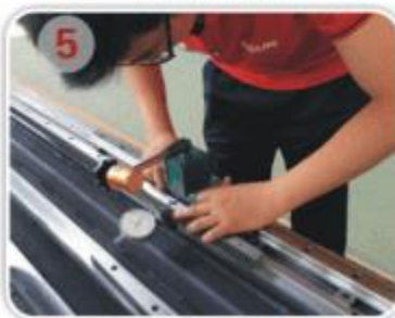
Flatness: using plug gauge to check the rack and gear
