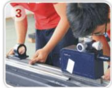
Straightness: using auto collimator to check frame
