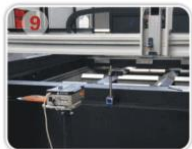
Precision: using interferometer to check X/Y stroke
